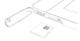
To eject the card, slightly press on its edge until it will be unfixed, and pull it to get.
