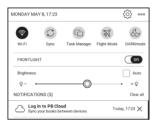
Notification panel gives an easy access to configuration of <u>Wi-Fi, Task Manager, Flight Mode, Sync, DARKmode</u> of network services and <u>Frontlight</u>.
