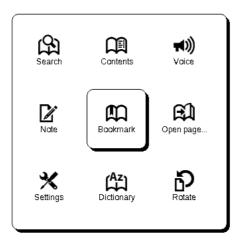
This menu can be brought up by 'OK' pressed in reading mode. The fast access menu content depends on a reading program (reader). Menu items:
