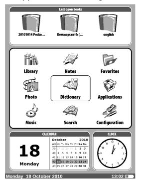
The Main Menu is a software element which displays basic functional and control sections for convenient use of the device:
